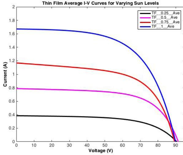
Figure 6. Comparison of average I-V curves at varying irradiance
