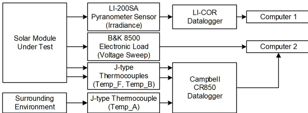
Figure 1. Block diagram of equipment connections.
